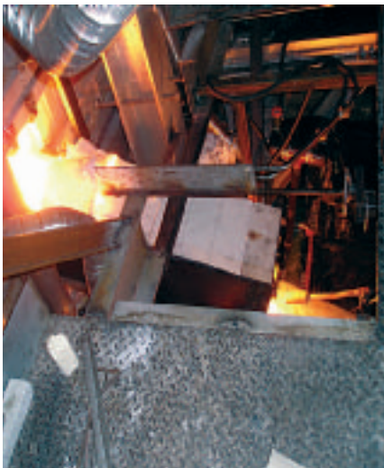
Typical location of the tapping hole and draining of the furnace.
